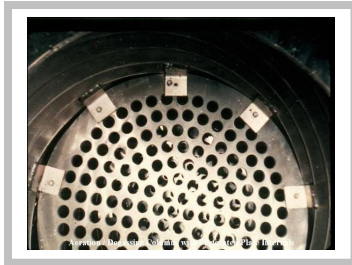
Figure 5-4 - Diffuser Used for Bubble Aeration
