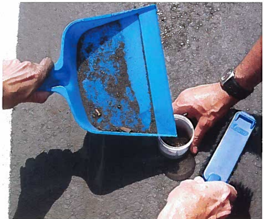
Figure 3: Dust swept from pavement with coal-tar-based sealcoat contains very high concentrations of polycyclic aromatic hydrocarbons (PAHs).
